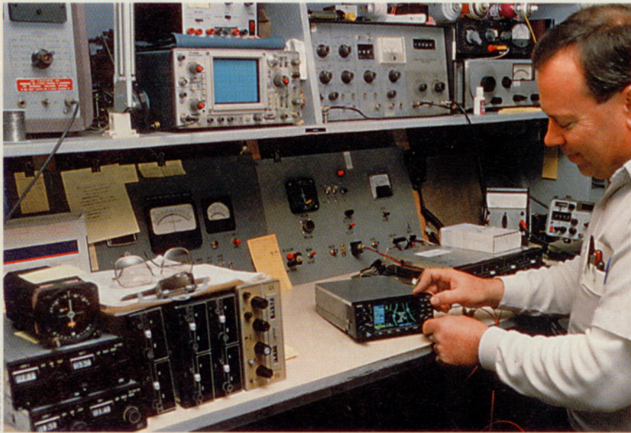
Fabricated panels are test-fit before being sent out for finishing (top). It's this stage—filling and trimming and making sure the clearances are just so —that consumes so much time. Randy Kiesz (above) puts the Garmin GNS 430 through a burn-in on the bench; all of the major avionics were pretested this way.
